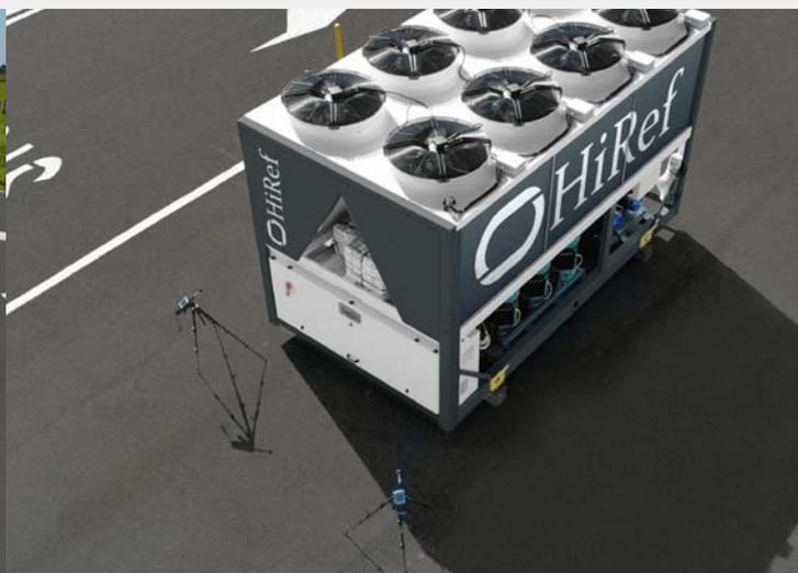
HiRef ensures a minimum accuracy range for all measurements in accordance with the UNI EN 14511-3 standard. The instruments are subject to rigorous checks at regular intervals to ensure they are properly calibrated at all times. In addition, the entire measurement chain is fine-tuned during calibration of each instrument.
