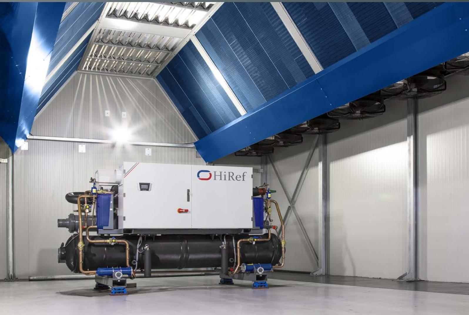
A recent addition, the **Hyper Lab** was entirely designed and built by HiRef's R&D department to test air-to-water and water-to-water chillers and heat pumps as well as large-sized (HiRef DataBatic) and high power (up to 1.5 MW nominal cooling capacity and 2.0 MW heating capacity) air-to-air units. For air-to-air units, the lab can simulate an external environment (outside air intake) with temperatures as low as  $-35\text{ }^{\circ}\text{C}$ .
