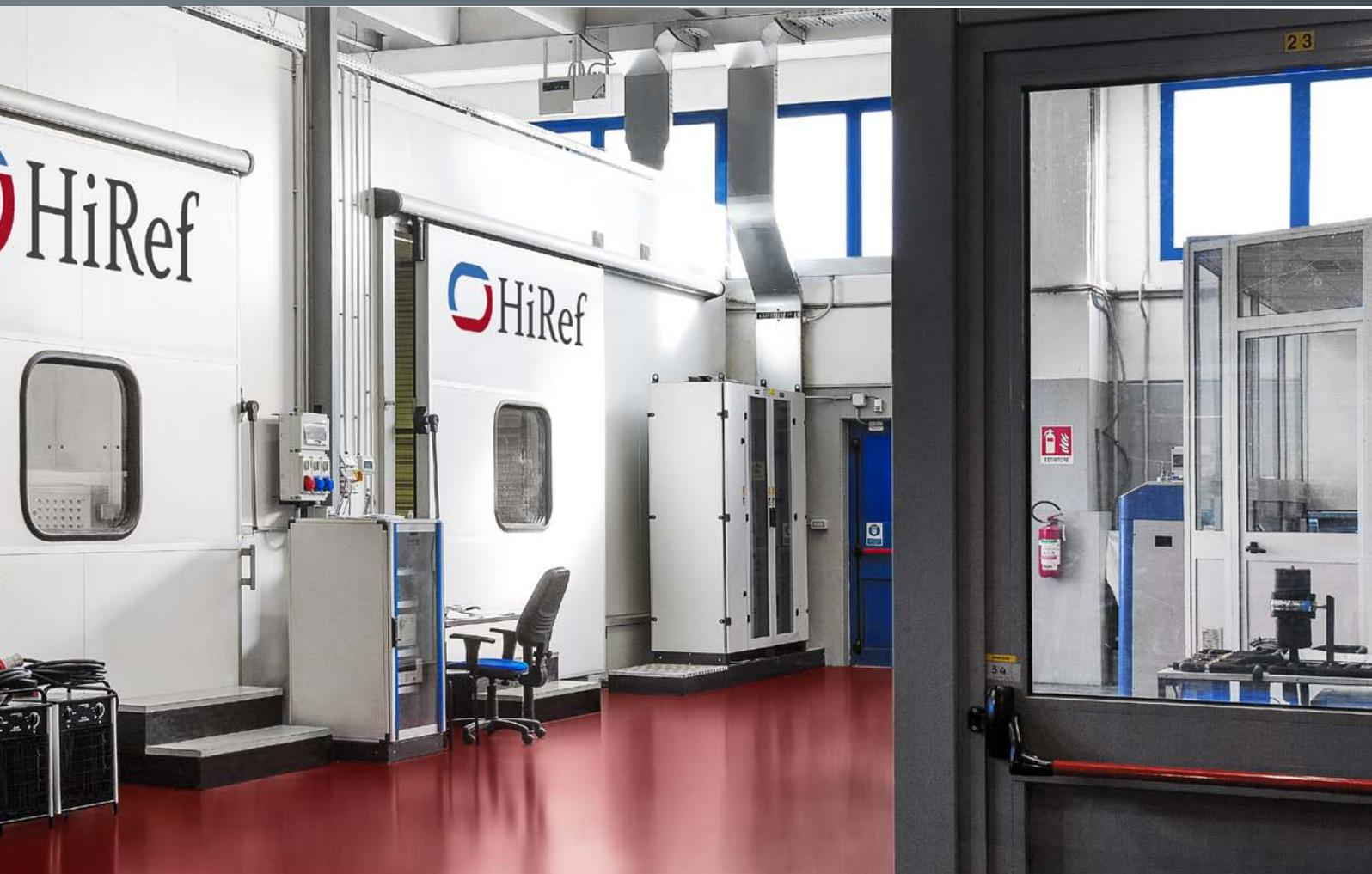
**Data Centre Lab** is a climatic laboratory with raised floor and false ceiling used to replicate different server room layouts. The infrastructure enables us to test direct expansion or chilled water units and allows for reversible and multi-directional airflow inside the room to adapt to different test configurations. With the Data Centre Lab we can exactly reproduce actual operating conditions to test CRAC units with Upflow, Downflow or Displacement configuration.
