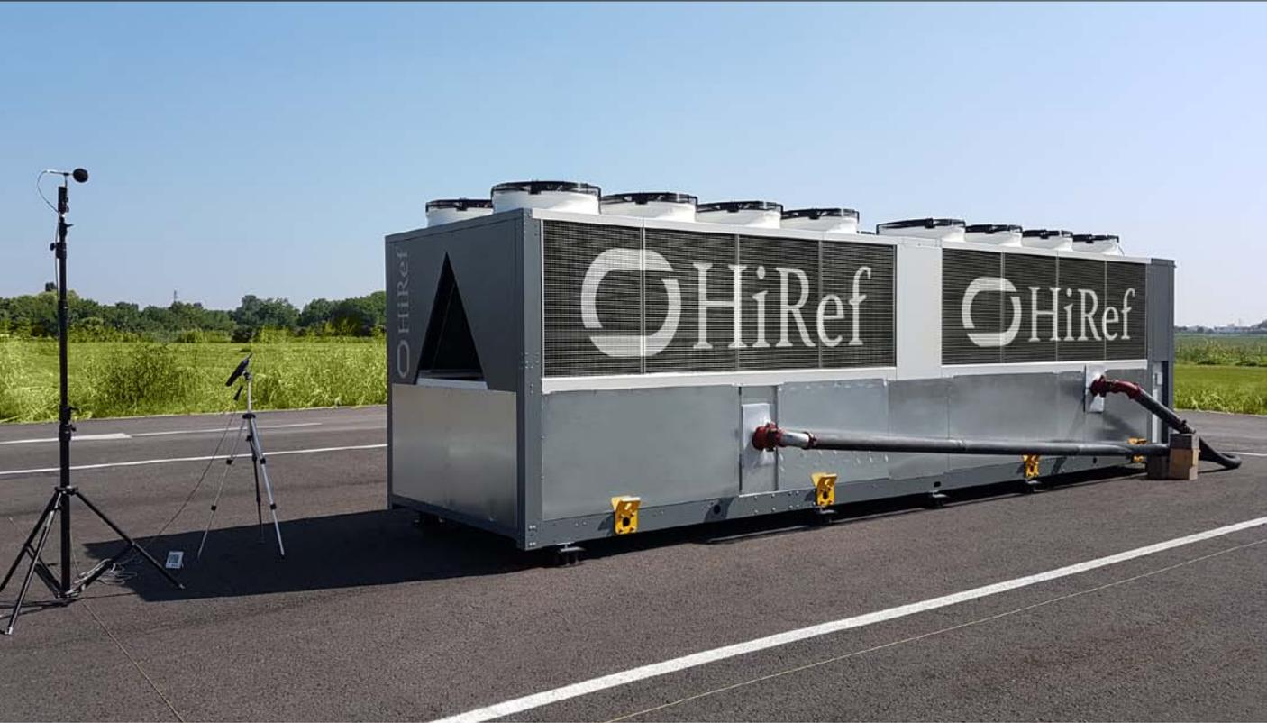
Thanks to our collaboration with the University of Padua, we can draw on the expertise of academics for the certification of acoustic tests performed in an off-site qualified area compliant with the UNI EN ISO 3746 standard. Class 1 instruments are used, providing an accuracy of 1.5 dBA under favourable environmental conditions.
