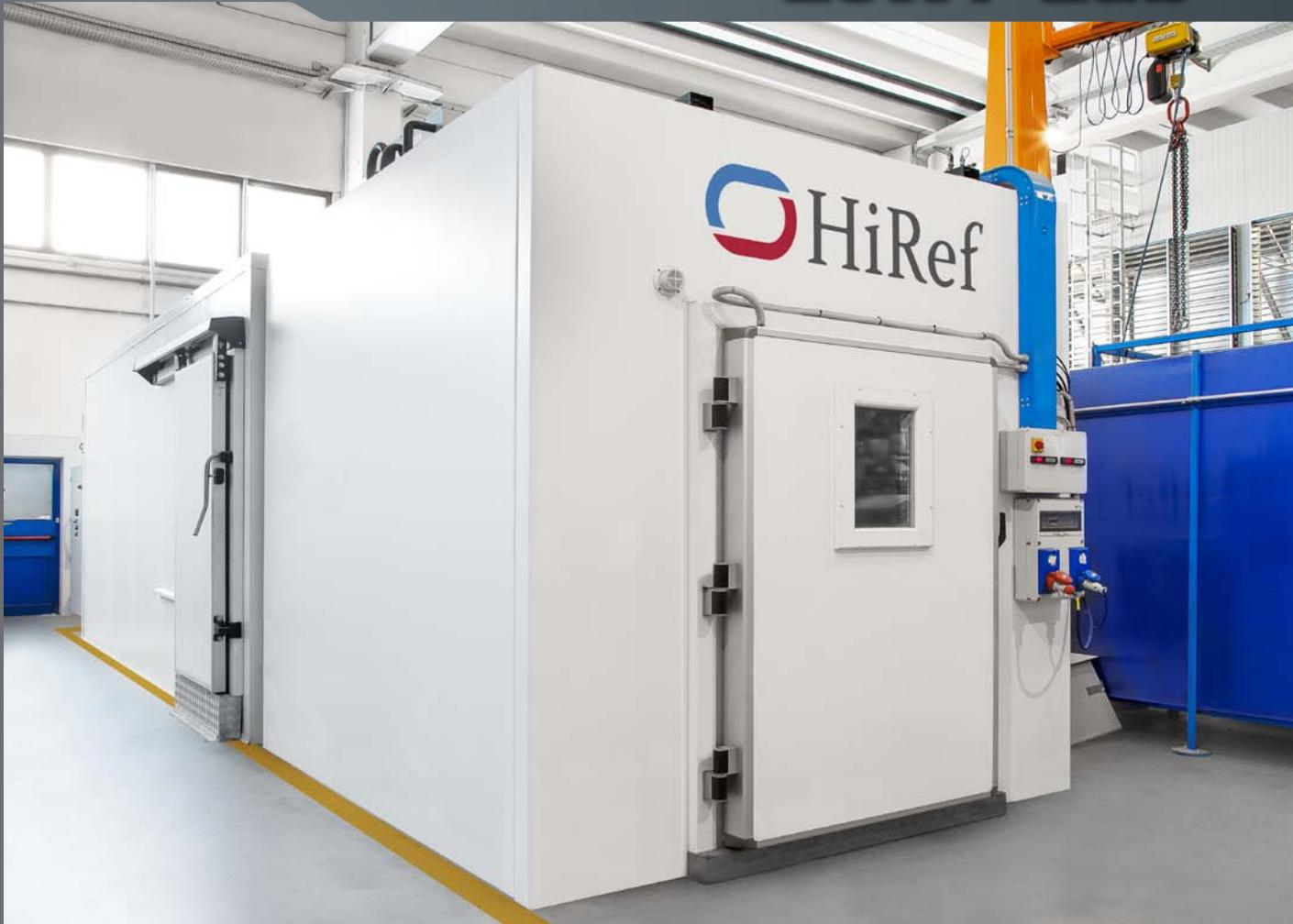
The **LowT Lab** is a climatic room used to recreate extreme temperature conditions (as low as  $-50\text{ }^{\circ}\text{C}$ ), simulating the coldest winter climates. This makes it possible to test monobloc telecom air conditioners; components such as test units, fans, and electrical panels; and reduced-scale prototypes. To maintain critical temperature conditions, the room uses direct expansion units connected to a two-stage compressor with sub-critical  $\text{CO}_2$  refrigeration cycle.
