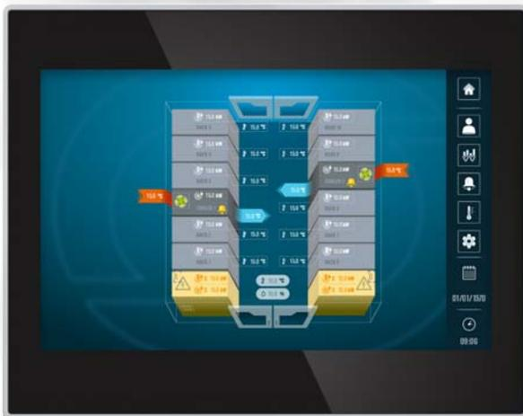
The user can interface with the control system via a **13" touch display**, which can be installed on-board the island - if the customer orders the island aisle door in its automatic version - or mounted on a *stand-alone case*.
