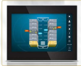
The user can interface with the control system via a 13" touch display, which can be installed on-board the island - if the customer orders the island aisle door in its automatic version - or mounted on a *stand-alone* case.
