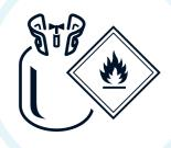
Safety ASHRAE A2L class refrigerants are mildly flammable. This peculiarity requires certain precautions in terms of sensors and components in the air conditioning unit, to prevent through adequate designing - the risk of igniting fires.
